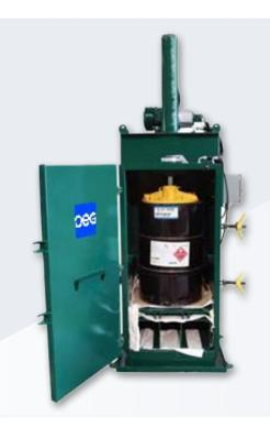
OEG's **ENVIRO**PAK drum crushers compact waste into 55 - 85 gallon drums before crushing the waste further. The Drum crushers can compact 55 gallon drums to 4" and reduce disposal costs of hazardous waste by compacting into UN/DOT approved drums. All units meet and exceed international MARPOL 73/78 Annex V and utilise UL listed components.
