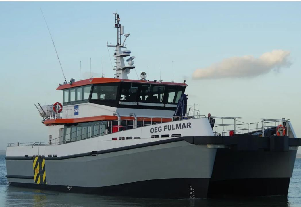
Fulmar is a multi-purpose offshore crew transfer vessel designed to transport personnel and equipment to and from offshore wind farms.
