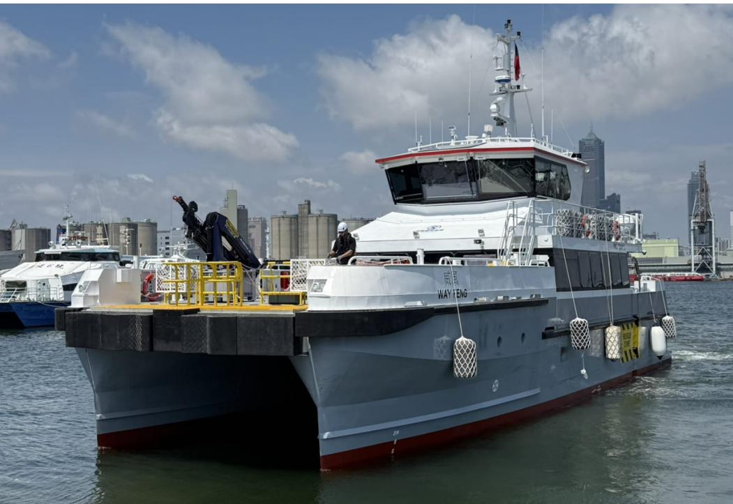
Way Feng is a multi-purpose offshore crew transfer vessel designed to transport personnel and equipment to and from offshore wind farms.
